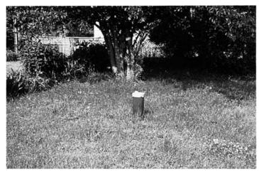
Note 1—Photograph shows an approximately 8-in. diameter outer well casing in the yard of a home. Releases of chemicals or petroleum products near or into a well can result in the contamination of the groundwater aguifer in which the well is constructed.
